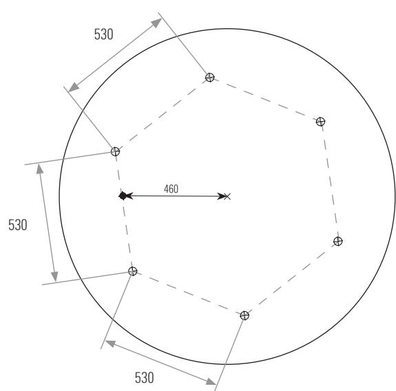
◆ POWER ENTRY      ◇ SUSPENSION MOUNTING SCREW and MOUNTING HOLE
